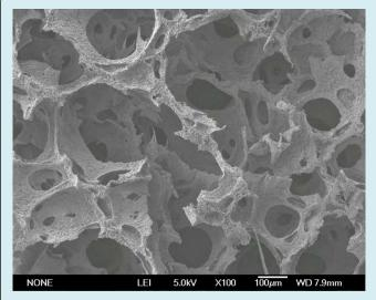
**Figure 1:** SEM morphology of the new polyvinyl alcohol foam material via air-foaming process(x100).
