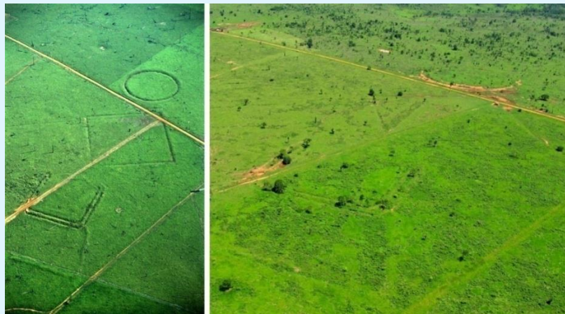
Figure1: Aerial remote sensing is a useful method to monitor the degradation of archaeological sites, as well as other changes in the landscape. As an example are the images of the Fazenda Colorada site, photographed first in 2002 and again 9 years later, in 2011. The processes of earthwork decay and erosion are clearly visible.
