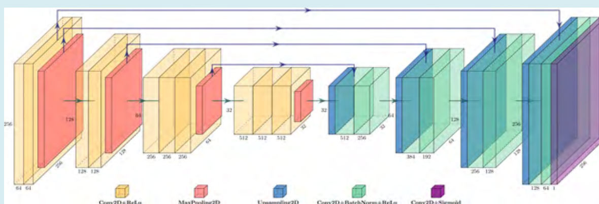
Figure S1: Architecture of the computer vision model. Planes represent hidden unit arrays, and arrows represent connections between the units. Yellow and red blocks represent a VGG16-backbone encoder part with weights pre-trained on Image Net dataset. The blue, green, and purple blocks represent a custom decoder part. Note U-Net-like skip connections.
