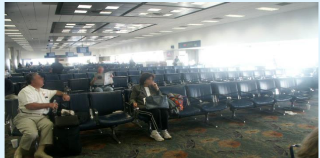
Figure 1: Example of daylight glare and sunlight heat gain at an airport boarding gate.
