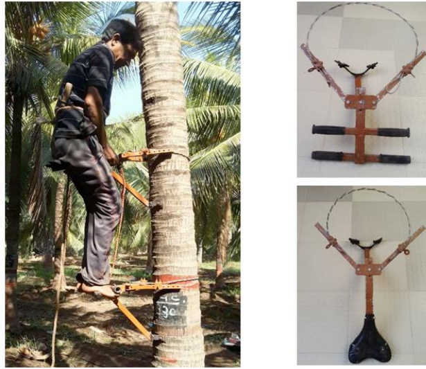
Figure 4: Sitting type coconut palm climbing device.
