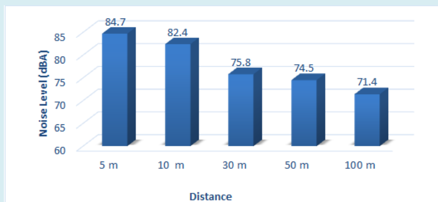
Figure 2.2: Noise Levels w.r.t. with Distance from Right Side Boundary on Double Hammer, Trimming Machine, Grinders, Coining Machine and Blank Cutting Machine.
