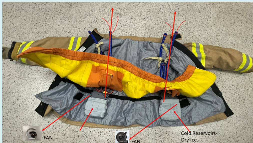
Figure 1: The LC coat made up of carbon nanotube-based fabric inside with two pouches and a fan. Components of the coat are indicated by arrows.
