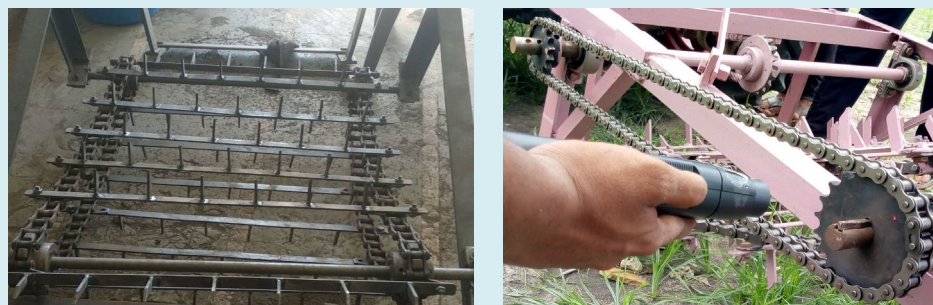
Figure 3: Fabricated elevator and power transmission.
