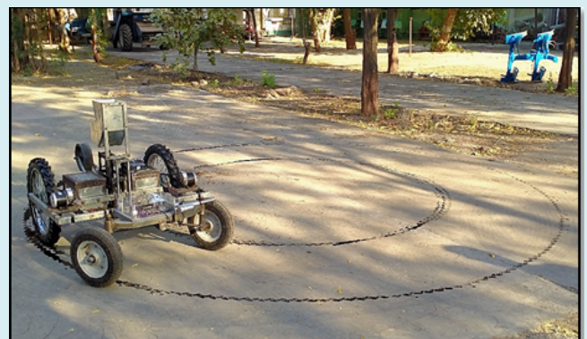
Figure 8: Determination turning radius of unmanned remote control agricultural vehicle.
