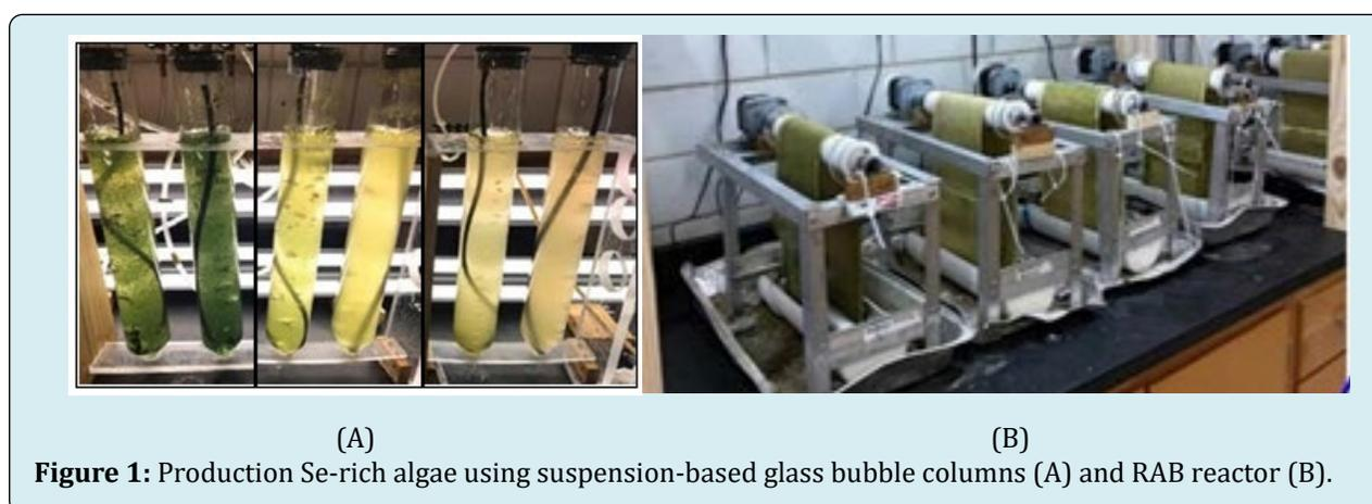
**Figure 1:** Production Se-rich algae using suspension-based glass bubble columns (A) and RAB reactor (B).
