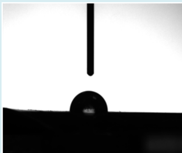
Figure 7: Contact angle of PVDF membrane.
