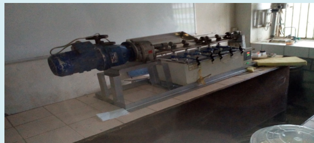
Figure 1: The fermentor used for liquefaction and Saccharification.
