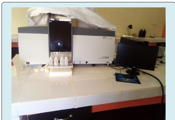
Figure 1: An atomic absorption spectrophotometer instrument in the laboratory.
