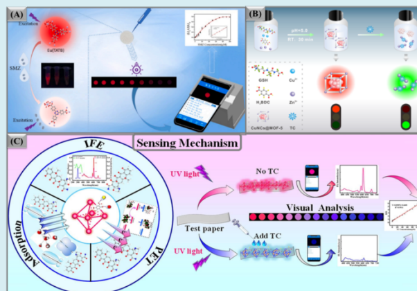
Figure 3: ANBs residue recognition based on the fluorescence-based sensing assays; (A) Eu-Ln-MOF complex for SMZ (16), (B) CuNCs@MOF-5 complex for TTC (13), and (C) \text{Ag}^+/\text{Eu}^{3+} @MOFs for TTC [26].
