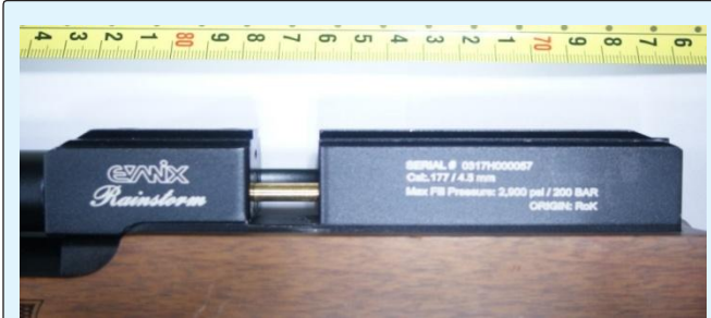
Figure 2: The serial number, the visible calibre and the max fill pressure of the Evanix, Rainstorm air rifle.
