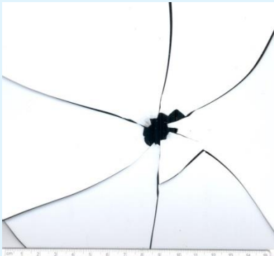
Figure 5: 8mm bullet entry hole 30".
