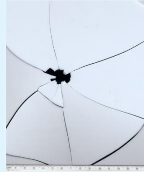
Figure 4: 8mm bullet exit hole 27".
