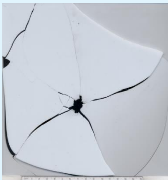
Figure 7: 8mm bullet entry hole 19".
