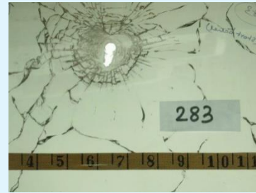
Figure 23: 8mm bullet exit hole on glass sheet.
