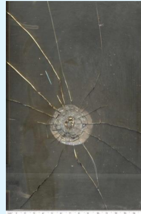
Figure 20: 5.56mm bullet exit hole on 2' Glass sheet on 2' glass sheet.
