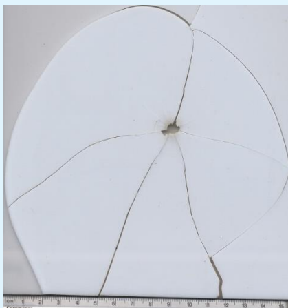
Figure 13: 8mm bullet entry hole 18''.
