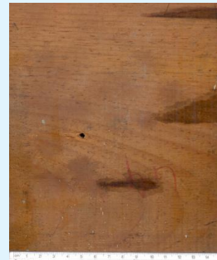
Figure 25: 5.56mm bullet exit on wood hole 26" on wood.
