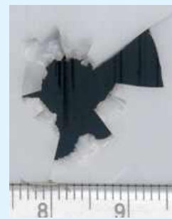
Figure 10: .303" bullet exit hole 21".
