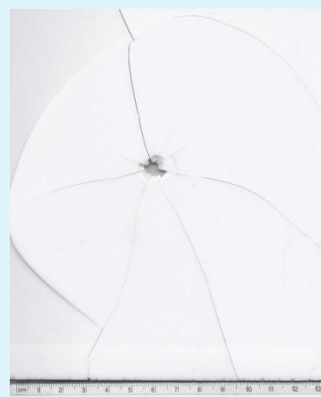
Figure 14: 8mm bullet exit hole 18''.
