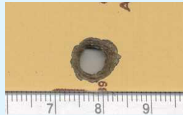
Figure 18: 8mm bullet exit 27.5" on Bakelite hole 27.5" on Bakelite. (Close up view)
