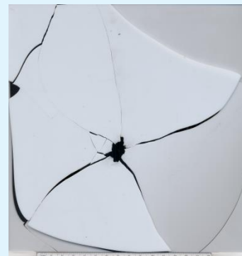
Figure 2: 8mm bullet exit hole 27".
