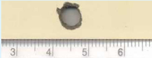
Figure 17: 8mm bullet entry hole. (Close up view)
