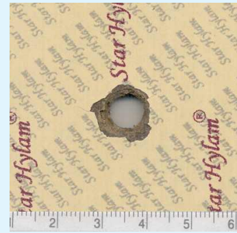
Figure 12: 8mm bullet exit hole 21'' Bakelite sheet.
