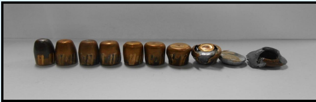
Figure 1: Showing extent of deformation in 9mm jacketed bullets on passage through iron sheets of gauges 30,28,26,24,22,20,18,16,14 respectively(from left to right). The bullet after passing through 2mm thick iron sheet (14 gauge) got separated between core (shaped as a disc) and jacket (along with some part of lead).
