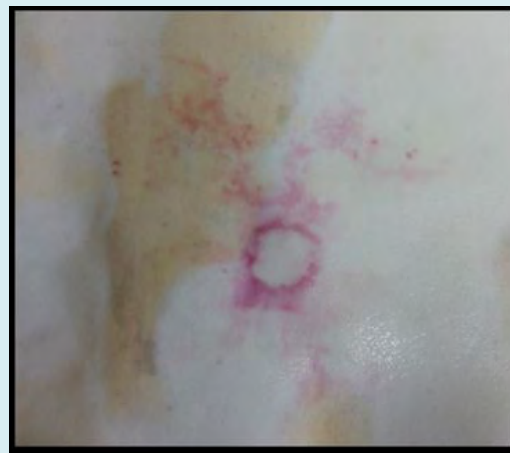
Figure (10b): figure showing positive detection of lead chips along with lead splash around bullet hole made by .22-inch calibre bullet on sheet of gauge 28.
