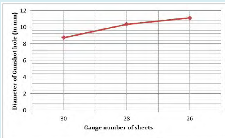
Figure 6: Showing increase in diameters of holes caused by .32-inch calibre bullets w.r.t gauge number of sheets.
