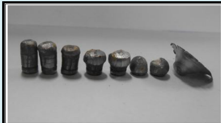
Figure 5: Showing variations in deformation of .22-inch calibre lead bullets when fired through iron sheets of gauges 30,28,26,24,22,20 and 18 respectively(from left to right). The core of lead bullets in form of pellets passed through sheet of gauge 20 and gauge 18 respectively. In gauge 16 sheet, the fired bullet was unable to penetrate and was found lodged in the target sheet (extreme right).
