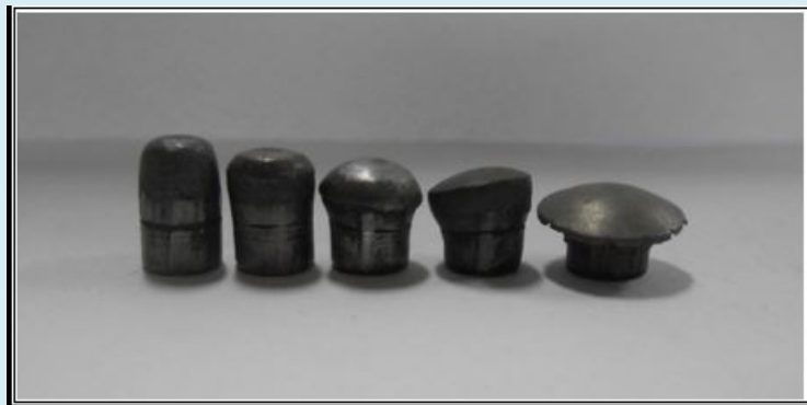
Figure 4: Showing extent of deformation in .32-inch calibre lead bullets on passage through iron sheets of gauges 30,28,26,24,22 respectively (from left to right).
