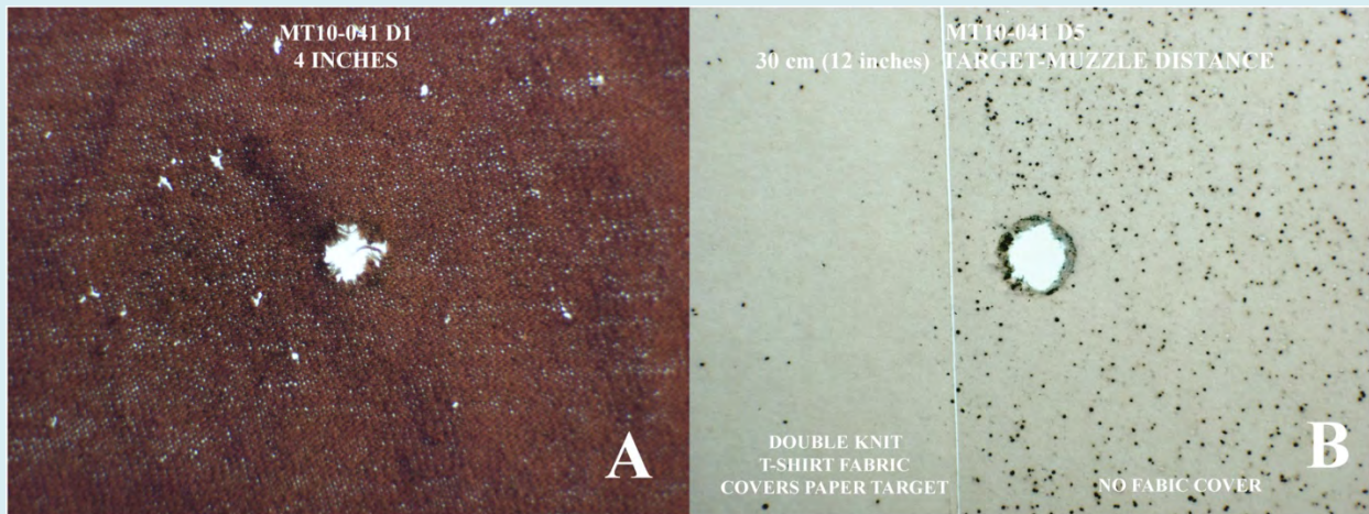
Figure 5. A. Backlit test fabric shot with the .357 caliber revolver muzzle 4 inches (10 cm) from the fabric; penetration of gunpowder fragments produced small holes around the bullet hole. B. The backlit target was shot at 12 inches (30 cm); the left part of the Benchkote material was covered with fabric, and the right part was uncovered. The gunpowder particles appear as dark stipples on the backlit paper. Most of the powder particles were prevented from penetrating the fabric, which covered the left part of the target.
