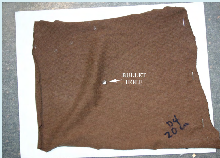
Figure 4. The test fabric was a worn t-shirt that was similar in weave and fabric thickness to Adam Owen's t-shirt; the test fabric was fastened over Benchkote paper [3], which was attached to plywood and then shot with the .357 caliber Hornady cartridges in the S&W revolver.
