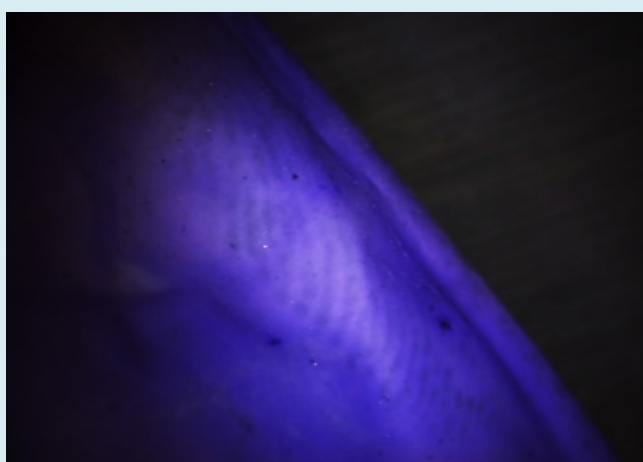
Figure 4: Gentian Violet Performed on Latex Gloves, Captured in a Stereomicroscope.
