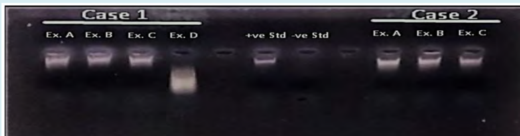
Figure 8:- The 1% Agarose gel electrophoresis results of isolated DNA Case-1 (Ex-A- Post mortem blood stain of suspected father, Ex-B- Dried umbilical cord of deceased baby, Ex-C- Blood stain of mother, Ex-D- Femur bone of deceased baby); “+ve” Std=20ng/l; “-ve” Std; Case-2 (Ex-A- Liquid blood of mother, Ex-B- Liquid blood of suspected father, Ex-C- Cord blood stain of the still born baby).
