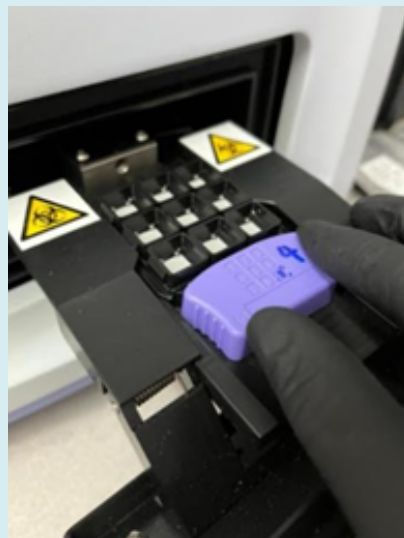
Source: Toxicology Laboratory - INACIF – 2022. Figure 3: Placement of Carrier Tray in the Equipment.
