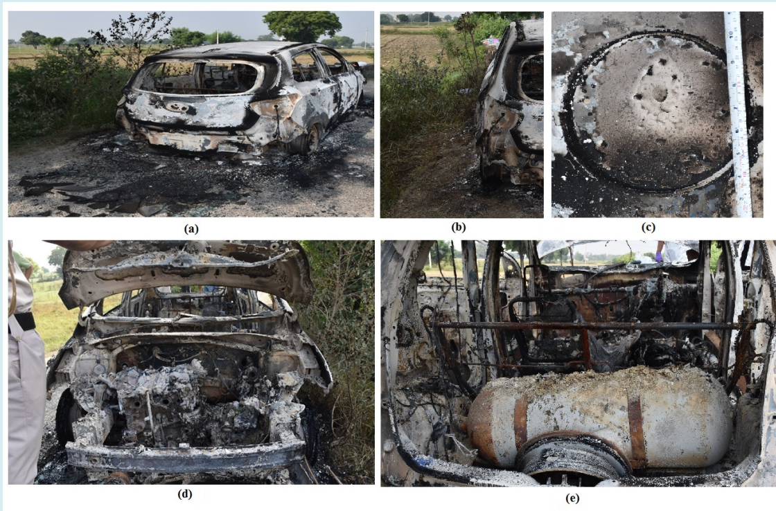
Figure 1: Illustrates (A) Metallic Frame or Remnants of A Completely Burnt Car with Smoke Lines & Soot Depositions, (B) Heating Effect on Plants Near Vehicle, (C) Unaffected Lid of Fuel Tank, (D) Completely Burnt Engine Portion of Car Exposing Wheel Rim, (E) Intact CNG Cylinder and Other Remnants of Car Seat View From Inside.
