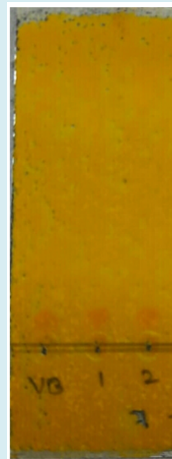
Figure 1: Thinlayer Chromatogram showing VB-Vecuronium control; 1- stomach & Intestine Samples; 2- injection-site skin puncture sample from left cubital fossa. (Solvent system-Chloroform: Acetone: Methanol = 7:2:1)
