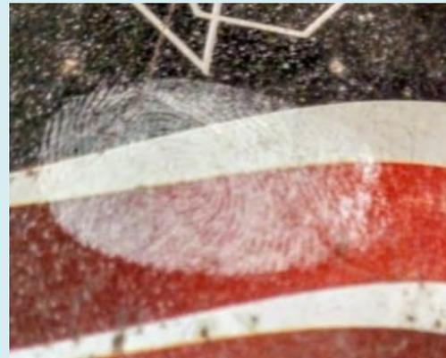
**Figure 5:** Development of Latent Fingerprint with the help of rock salt powder on Non-Porous Metal surface.
