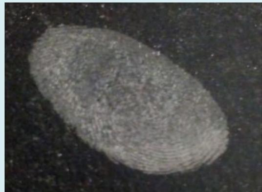
**Figure 6:** Development of Latent Fingerprint with the help of table salt powder on Porous CPU surface.
