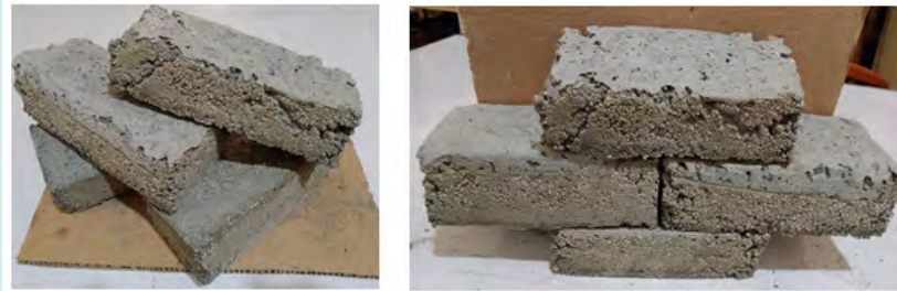
Figure 4: Lightweight bricks prepared from CKD and grated polystyrene waste and enhancing admixtures.
