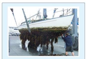
**Figure 2:** An evident invasion of marine benthos on a not managed ship hull).
