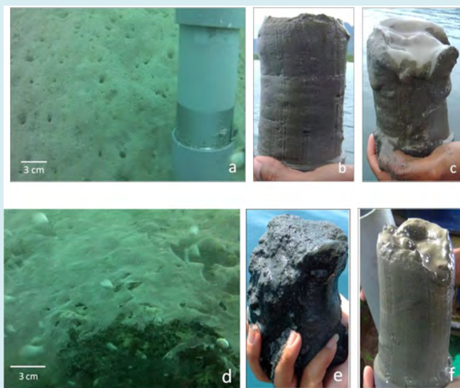
Figure 3: Typical sediment conditions at selected fish farms and reference locations: Seafloor (a) and sediment core (b) at reference location 12; sediment core at Fish Farm 18 (c); Seafloor (d) and sediment core (e) at Farm Cluster 21; sediment core at reference location 7 (f).
