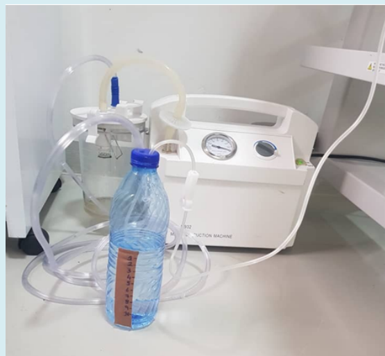
Figure 5: Infusion-giving set connected to our improvised underwater seal which was a 750ml water bottle; the tubing was inserted 2cm below the water line and bubbling with 2 tight holes in the plastic cap, an inlet (infusion set), and outlet. Bottle was kept upright on the floor, then another tubing (outlet) was connected suction machine at about -7.5cmH 2 O to complete the circuit.
