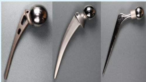
Figure 13: Cleaned metal parts of endoprostheses studied after being removed from patients during endoprosthesis replacement.
