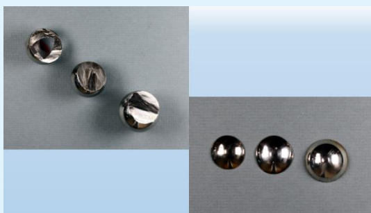
Figure 14: Fragments of cut heads of the endoprostheses. Left – view from the side of endoprosthesis; right – view from the side of the joint.
