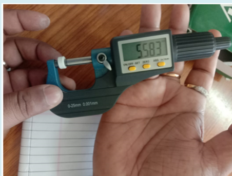
Figure 13: Thickness of Tablet.
