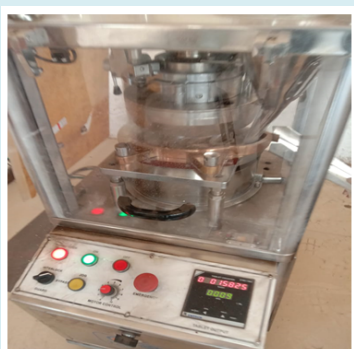
Figure 7: Automatic compression machine.
