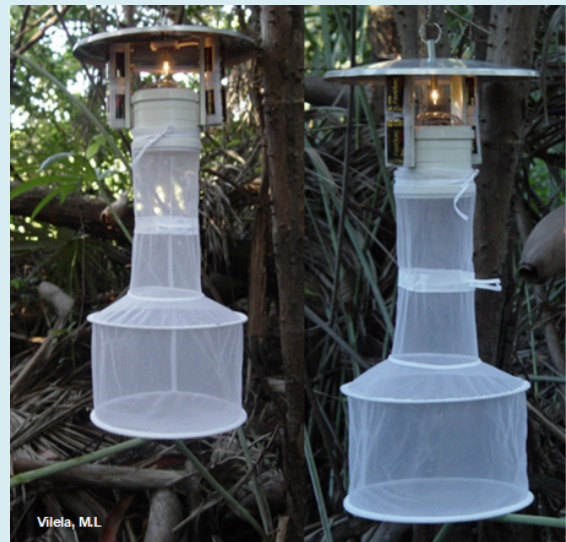
Figure 1: CDC traps with light bait, used to collect sandflies. At the researched location, the trap is placed from 6:00 pm until 6:00 am the following morning. Allowing for a more realistic description of the sandfly fauna and other insects in the region.
