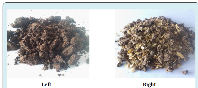
Figure 4: The Castor seed cake/shell mixture biomass (left) and the Neem seed cake/shell mixture biomass (right).
