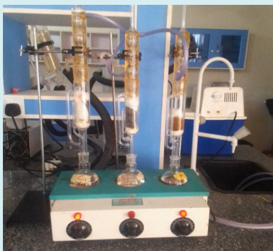
Figure 2: The Soxhlet extraction setup consisting of a heating mantle, boiling flask, sox let, and cold water condenser.
