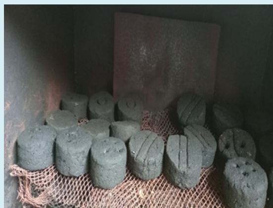
Figure 9: Briquettes drying in an oven.
