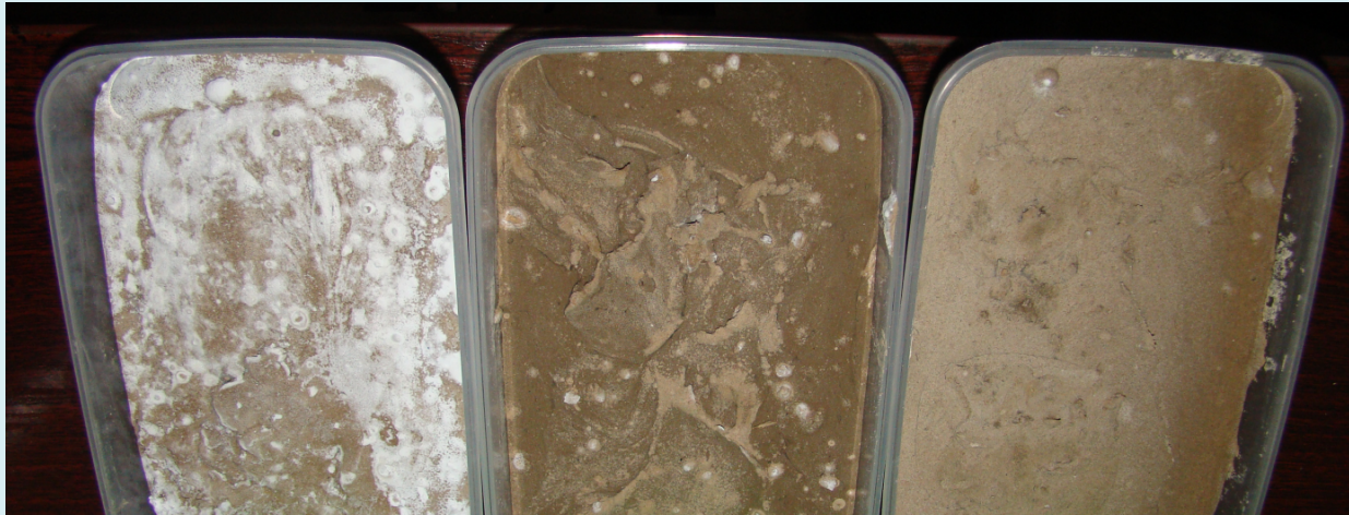
Figure 1: Samples with cement addition from left: 30%, 40% and 50%.
