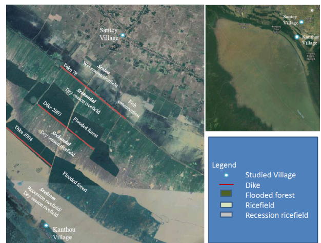
Figure 2: The Sre System, the Zoning and Block System for water management.
