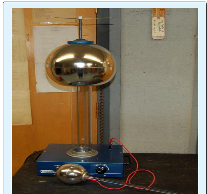
Figure 10: This demonstration shows that a pinwheel on a Van de Graff generator will spin [18].
