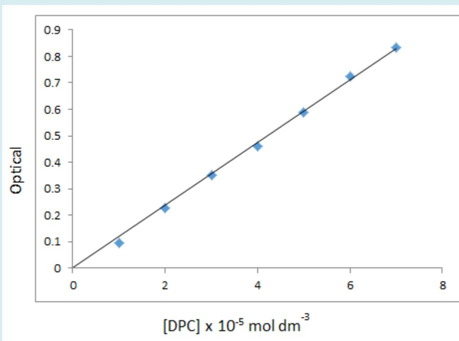
**Figure 3:** Verification of Beer's law for diperiodatocuprate (III) concentrations at 420 nm in aqueous alkali at 30°C.
