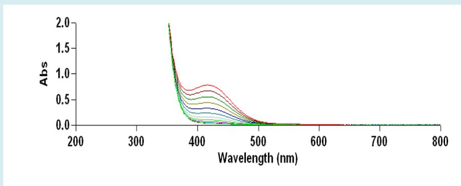
**Figure 2:** Spectroscopic changes occurring in the degradation of Enrofloxacin by diperiodato cuprate (III) at 25°C ([DPC] =  $3 \times 10^{-5}$ , [ENR] =  $1 \times 10^{-4}$ ).
