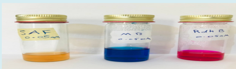
Figure 1: Prepared concentration of rhodamine B, methylene blue, and saffron dye.
