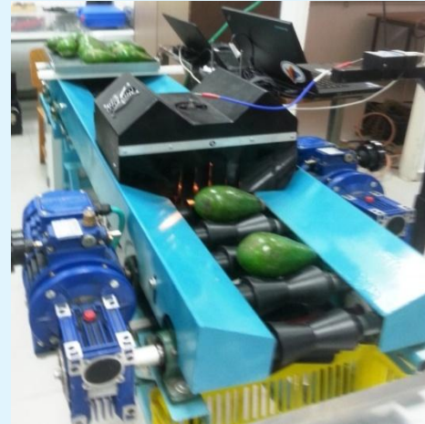
Figure 2: The new "grommet" developed in this study to improve the conveying track of non-spherical fruits such as avocado.
