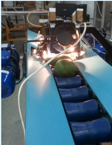
Figure 1: Measuring compartment on prototype of avocado sorting conveyor.
