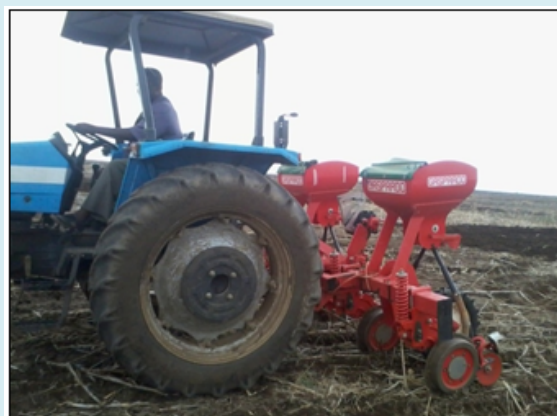
Figure 2: Zero tillage planter with double disk furrow opener.
