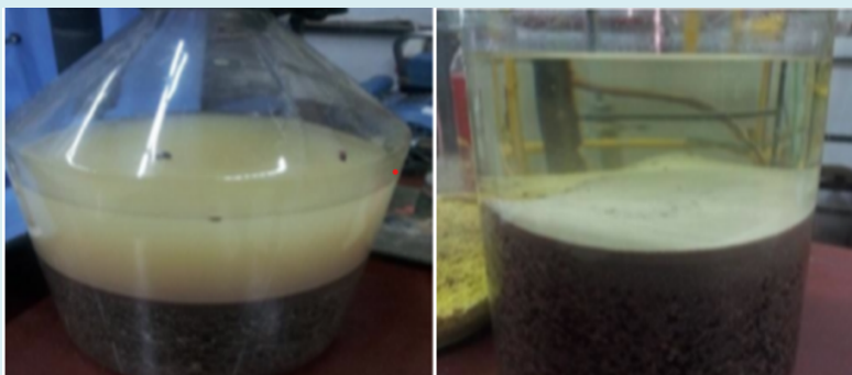
Figure 2: Solvent extraction of Baobab seeds oil with hexane and ethanol.
