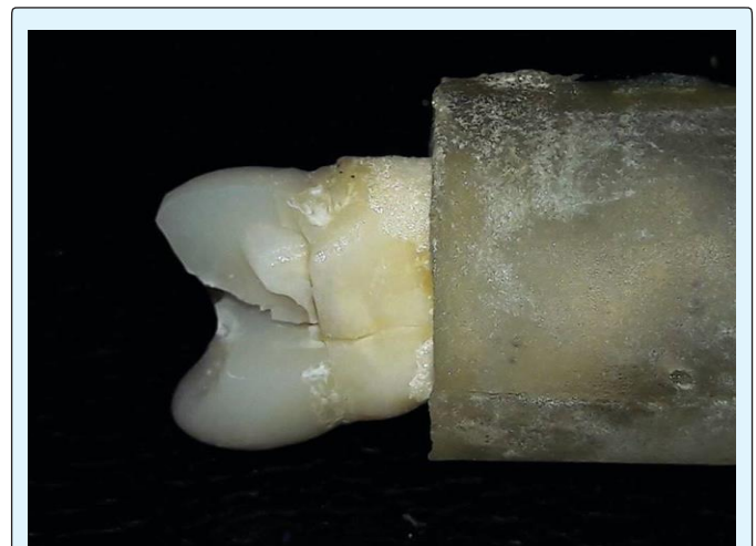
Figure 2: Digital image demonstrating catastrophic fracture (lava ultimate).
