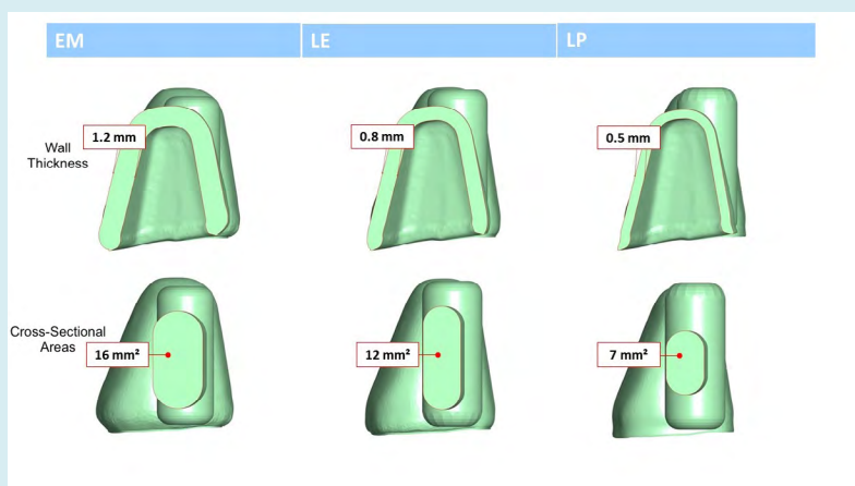
Figure 2: Wall thickness of the crowns were 1.2mm (EM), 0.8mm (LE), or 0.5mm (LP) with connector cross-sectional areas of 16mm 2 (EM), 12mm 2 (LE), or 7mm 2 (LP).
