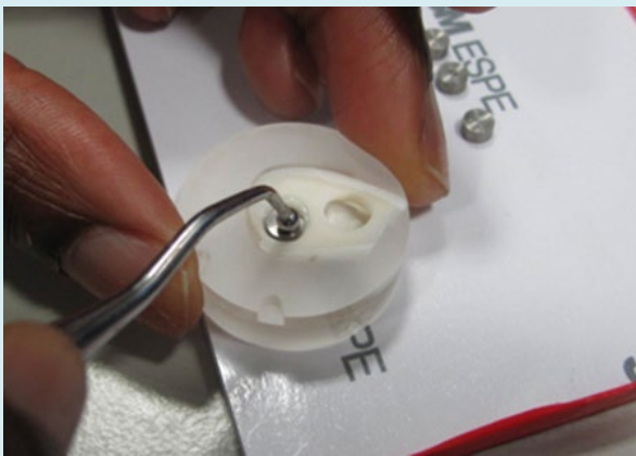
Figure 1: Stainless steel rod placed in prepared cavity contained with 30mg of resin cement.
