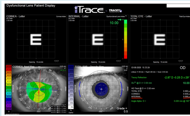
Figure 1: An example test result using one of the modules available in the iTrace analyser - Dysfunctional Lens Patient Display. It graphically shows how individual elements of the optical system, i.e. the cornea (top left) and the lens (top centre) and both elements together (top right) reproduce the quality of letter “E”, taking into account the HOA values generated by these structures. The HOA values are shown in numerical form below (bottom right). The value of HOA Internal generated by the lens is marked with a red line.
