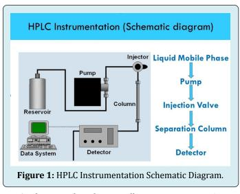
As shown in the schematic illustration in Figure 1 over, HPLC instrumentation [13,14] includes a pump, injector, column, sensor and integrator or accession and display system. The Main Part of the system is column in this separation occurs
