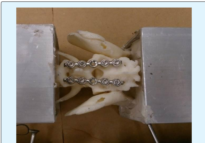
Figure 3: Instrumentation of the vertebral models. Vertebral models were plated with two 2.7mm SOP plates with five nodes. Each plate had two standard cortical screws placed in the pedicle of L7 and two screws in the body of the sacrum. The central node was left empty.
