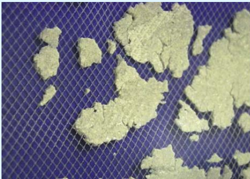
Figure 4 (c): Accumulation of Scale on Brine Spacer.
