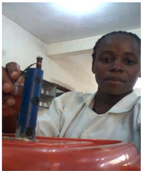
**Figure 4:** Fitted electrodes in the SMFC.
