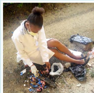
**Figure 1:** Harvesting graphite from 1.5V dry cells.
